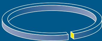
Butt joint: suitable for direct forming
