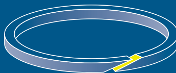
Scarf joint: unsuitable for direct forming
