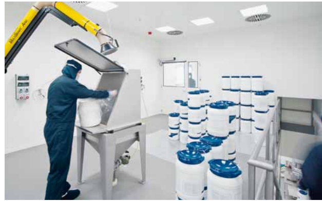
Loading station in the upper floor of the clean room
